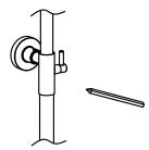
Step 5 Makesure the riser is level, mark the position of the screw holes.
